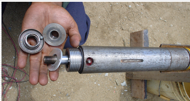
Core orientation device attached to wireline core barrel
