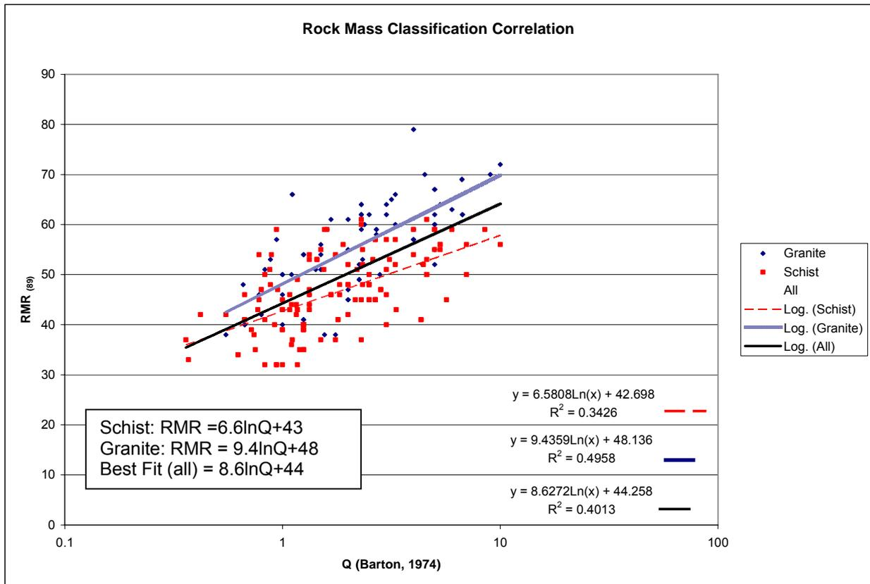
Figure 4: Site specific rock mass classification correlation for 7 Line Project.
