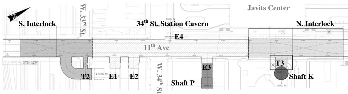
Figure 1: Plan view of 34<sup>th</sup> Street Station cavern along 11<sup>th</sup> Avenue showing the penetrations for future entrance development. Primary construction access was through Shaft P.
