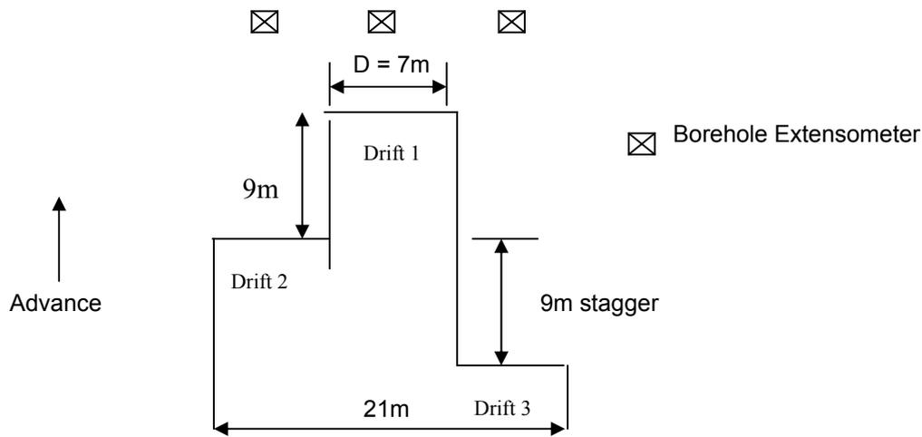
Figure 5: Plan of cavern top heading construction sequence and instrumentation arrangement.
